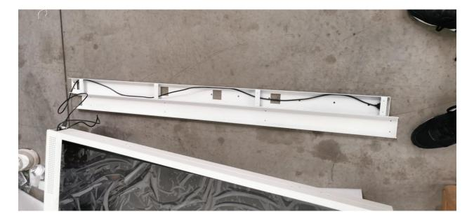
At this point also feed the black cable provided through one of the arms to the lowest square hole and pull it through.
